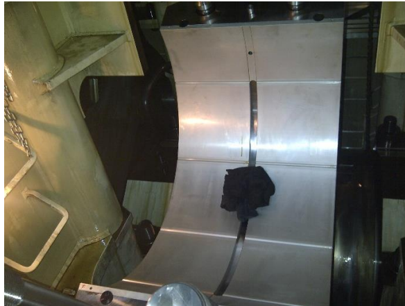
Breakdown analysis Investigation and Supervision during crosshead bearing shell replacement for MAN-B&W 9K90MC-C, (Hong-Kong)
